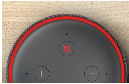
Fig. 1. Amazon’s button to turn off the microphone and the red-illuminated ring as an indicator [ www.amazon.com/Alexa-Privacy-Hub ] (Color figure online)
