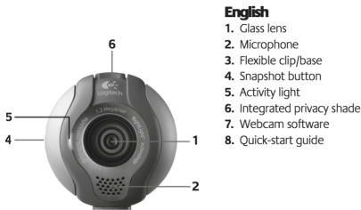
Fig. 4. Physically closable lid, denoted ‘6. Integrated privacy shade’, serves as both (a) physical kill switch and (b) indicator for Logitech’s webcam from 2009 [download01.logitech.com/24391.1.0.pdf]
