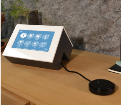
Fig. 2. External disconnect-able microphone serves as both (a) physical kill switch and (b) indicator; taken from the Candle IoT project [ www.candlesmarthome.com ]
