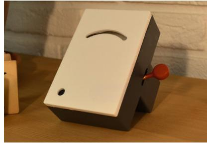
**Fig. 3.** Big red handle serves as both (a) physical switch and (b) indicator for the Candle IoT project’s carbon sensor [[www.candlesmarthome.com](http://www.candlesmarthome.com)] (Color figure online)
