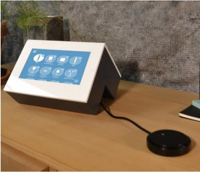
**Fig. 2.** External disconnect-able microphone serves as both (a) physical kill switch and (b) indicator; taken from the Candle IoT project [[www.candlesmarthome.com](http://www.candlesmarthome.com)]
